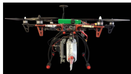
Figure 1: AA.DRL Student group Quadrants: Doguscan Aladag, Juan Montiel, Tahel Shaar, Vincent Yeh. Supervisor: Robert Stuart-Smith. Studio technical consultants: Tyson Hosmer, Manos Matsis, Multicopter with 3D-Printer hardware attachment
